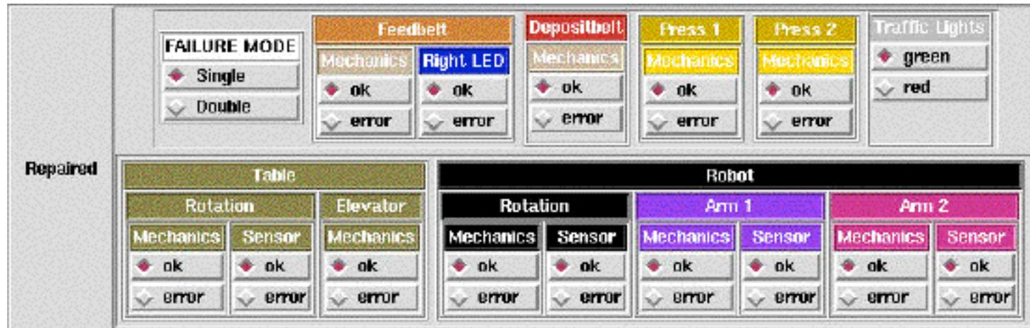
Single faults and multiple concurrent faults, of many different types, can be injected via this on-screen control panel
