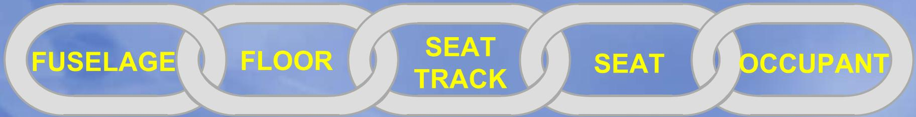
**Failures mostly in early links of the tie-down chain**
