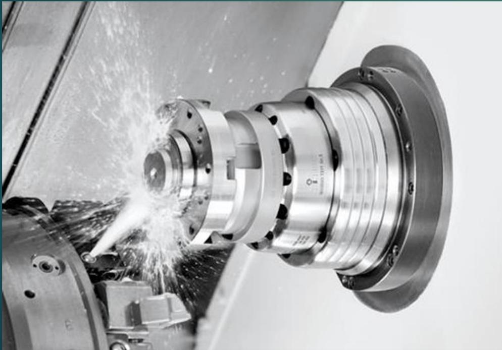
**Cutting oils** provide excellent lubrication properties for metal removal as well as chip evacuation from the cutting zone.
