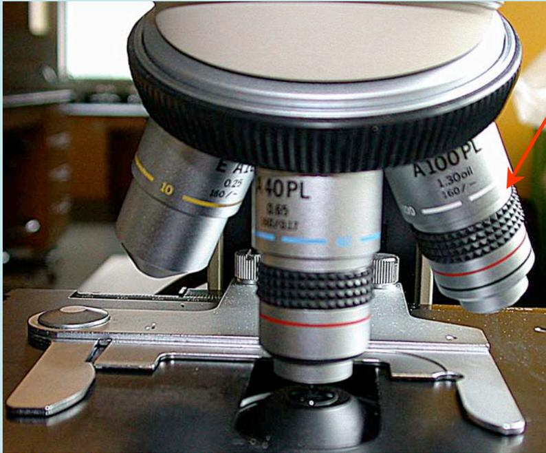
The 100X objective is an oil immersion lens. This means that in order for it to focus there needs to be a drop of oil between it and the coverslip of the specimen.
