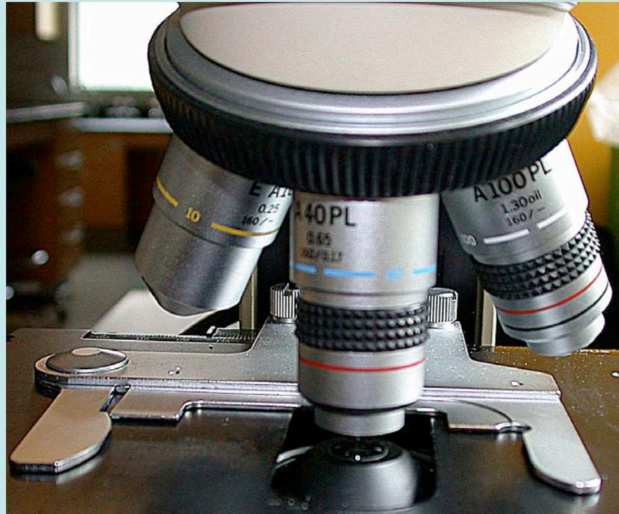
**WARNING** - once you have put oil on the slide you can not move back to the 40X lens. If you do, it will get oil on the 40X lens and will ruin the focus on it until it is cleaned. You can, however, rotate to the 10X or 20X lens. **Because of this problem it is best to use the oil immersion lens when you are completely done using the 40X on the specimen.**
