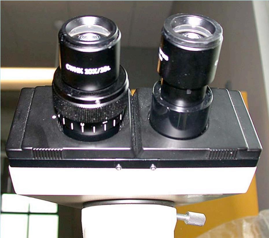
The oculars (eyepieces) on a binocular microscope should be adjusted to your interpupillary distance. Slide the the oculars until the distance is right for your eyes.
