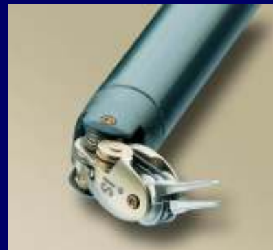
Endowrist ® Instrument which duplicates the dexterity of the surgeon
