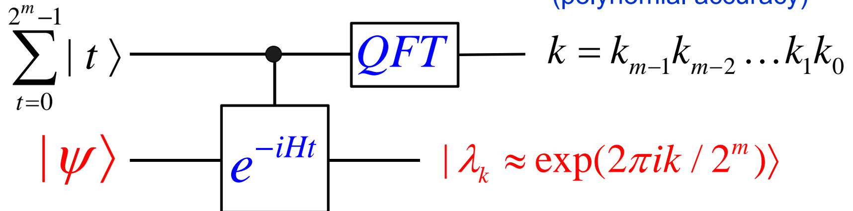
For a local Hamiltonian, measuring the energy to accuracy  $1/\text{poly}(n)$  is quantumly easy. We could measure the ground state energy if we could prepare a state whose overlap with the ground state is only polynomially small.
