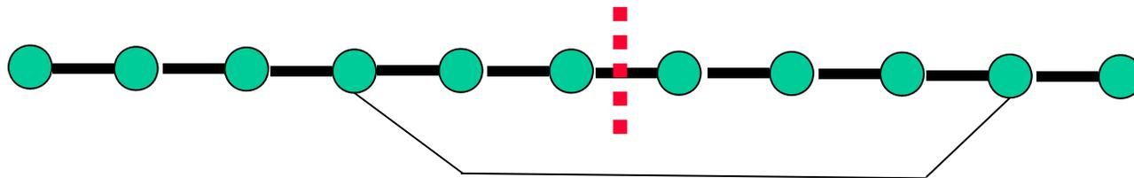
Arrange  $n$  qubits on a line. The initial state is a product state, and for any cut into two sets, the number of gates acting across the cut is  $E$ . Then if  $E = O(\log n)$ , the state has a succinct classical description (as a “matrix-product state”) and the quantum computation can be simulated “efficiently” (Vidal 2003, Jozsa 2006).
