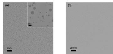
After 10-minute etching in H<sub>2</sub>O<sub>2</sub>/NH<sub>3</sub>, which dissolves WN but not Ru, (a) 1.3 nm Ru on 10 nm WN film showed many pinholes, but (b) 2.3 nm Ru on 10 nm WN film did not have pinholes.
