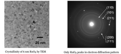
Crystallinity of 6 nm RuO<sub>2</sub> by TEM Only RuO<sub>2</sub> peaks in electron diffraction pattern
