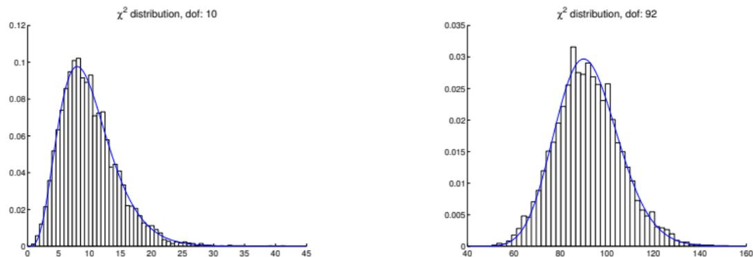
**Figure:** Normality check of the correlation integral vector by the  $\chi^2$  test for the Lorenz 63 system. Left: with 10 radius values used. Right: with 92 radius values
