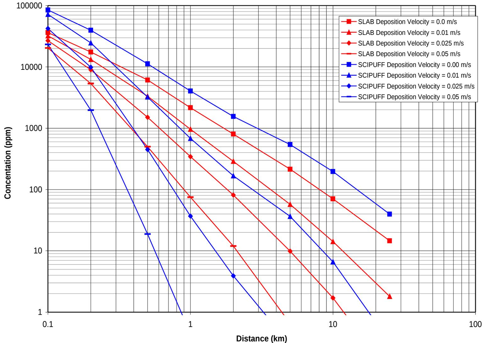
Modeled chlorine concentrations downwind of the hypothetical railcar release for the "base case", illustrating the effect of including deposition in SCIPUFF and SLAB simulations.
