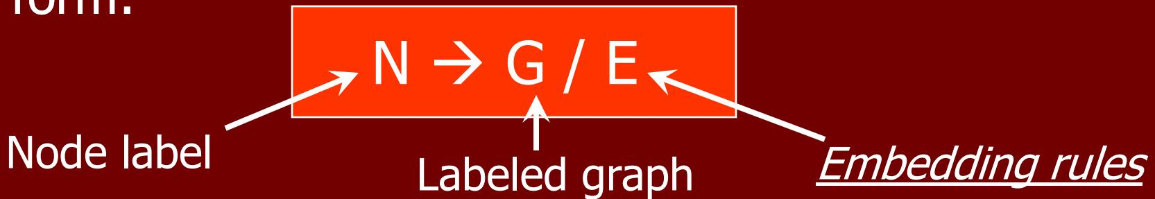
Replace any node with label  $N$  by  $G$ , connecting  $G$  to  $N$ 's neighborhood according to the embedding rules listed in  $E$ . *Embedding rules are based on node labels.*
