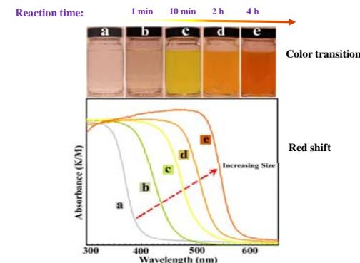
Optical images and UV-Vis spectra *E. coli*-templated CdS nanostructures in solution after (a) 0 min, (b) 1 min, (c) 10 min, (d) 2 h, and (e) 4 h of reaction.
