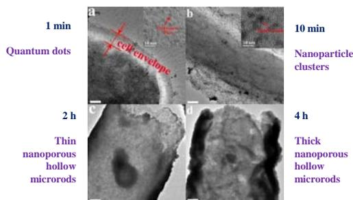
TEM images of *E. coli*-templated CdS nanomaterials synthesized as a function of reaction time. (a) Monodisperse quantum dots formed after 1 min; (b) near monodisperse nanocrystals formed after 10 min; (c) continuous nanoparticle agglomerates formed after 2 h; and (d) uniform porous coating formed after 4 h. All scale bars are 100 nm. The HRTEM images in the inset to (a) and (b) show more clearly the formation of quantum dots and nanocrystals, respectively.
