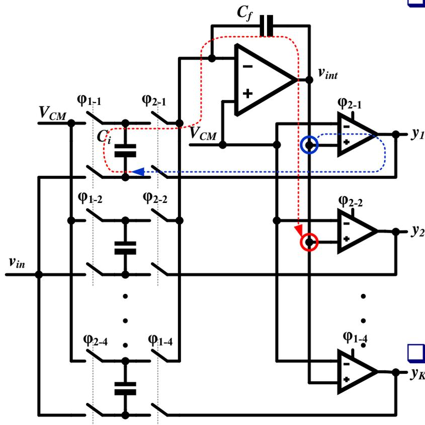
□ In order to achieve true first order noise shaping (K-times), the chain of noise differentiation should not be broken:
