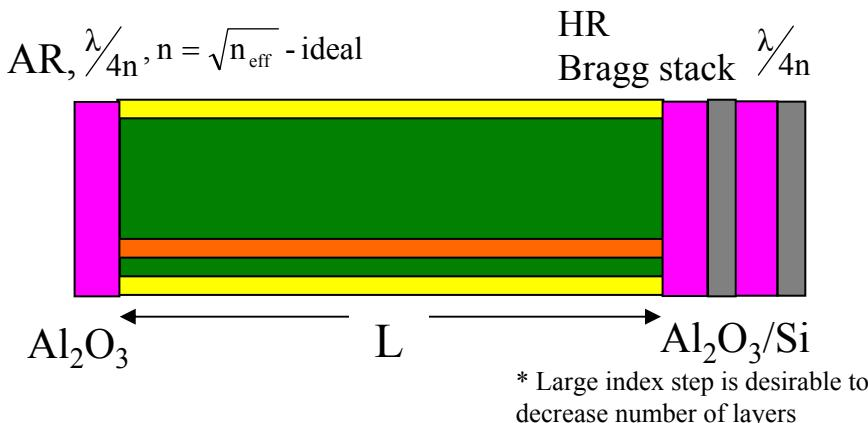
High power lasers are usually AR/HR (3-5%/95%) coated to direct all power to one mirror. The higher is the output power, the lower absorption coefficient the mirror coatings should have. Development of extra-low absorption optical coatings is now very important research direction due to numerous applications in solid state and semiconductor lasers industries.
