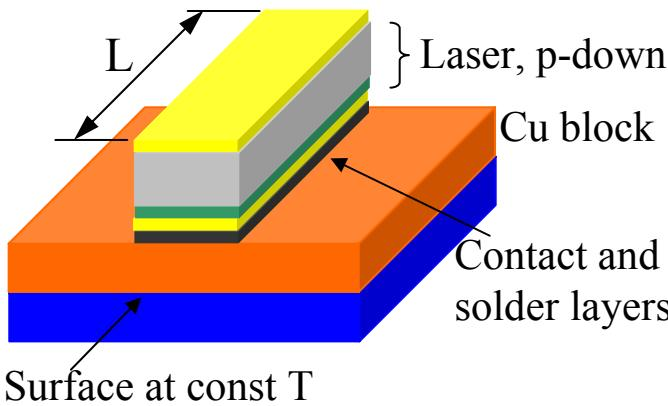
$$R_{TH} \propto \frac{1}{\text{cavity length, } L}$$
