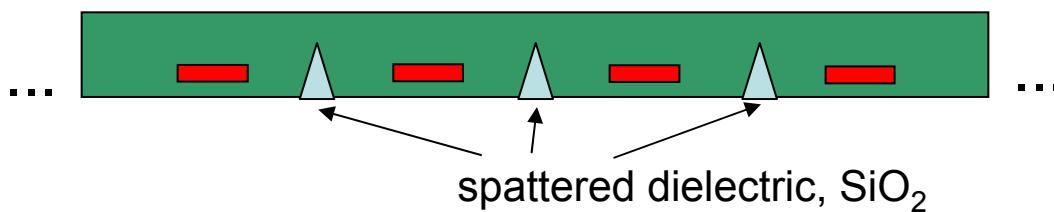
1D laser array is laser bar with emitters defined by metal contact stripes.
