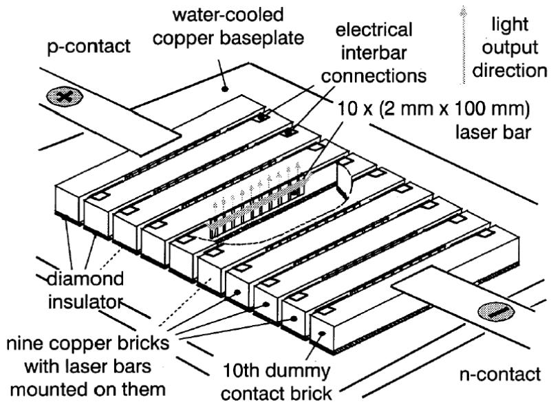
2D laser arrays can produce hundreds watt of CW output power. 2D arrays can be further combined into stacks of array and produce total power of >10kW in relatively compact package.
