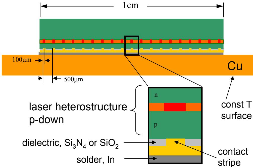
\* for large values of the bar fill-factor laser bar can become transparent in lateral direction and its output power will saturate. Spoiling lateral cavity grooves must be etched – additional processing step.
