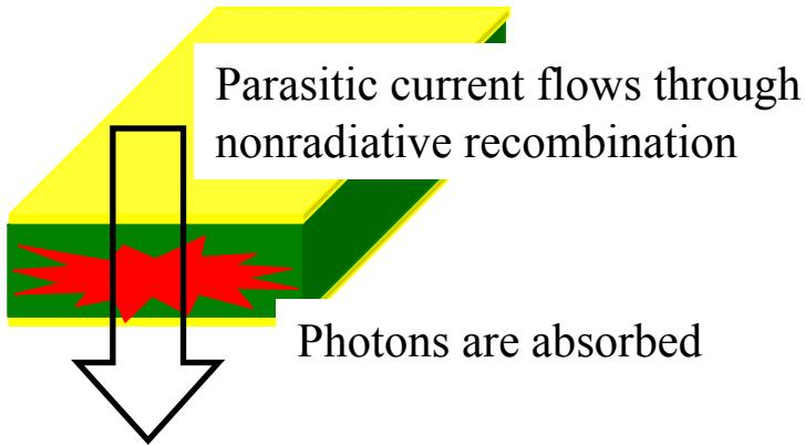
1. Nonradiative recombination on surface defects leads to slow mirror overheating proportional to laser operating current.
