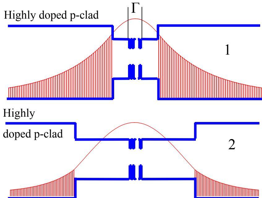
Confinement factor  $\Gamma$  for broadened waveguide devices is slightly reduced but the losses decrease dramatically resulting in net decrease of the threshold current density.
