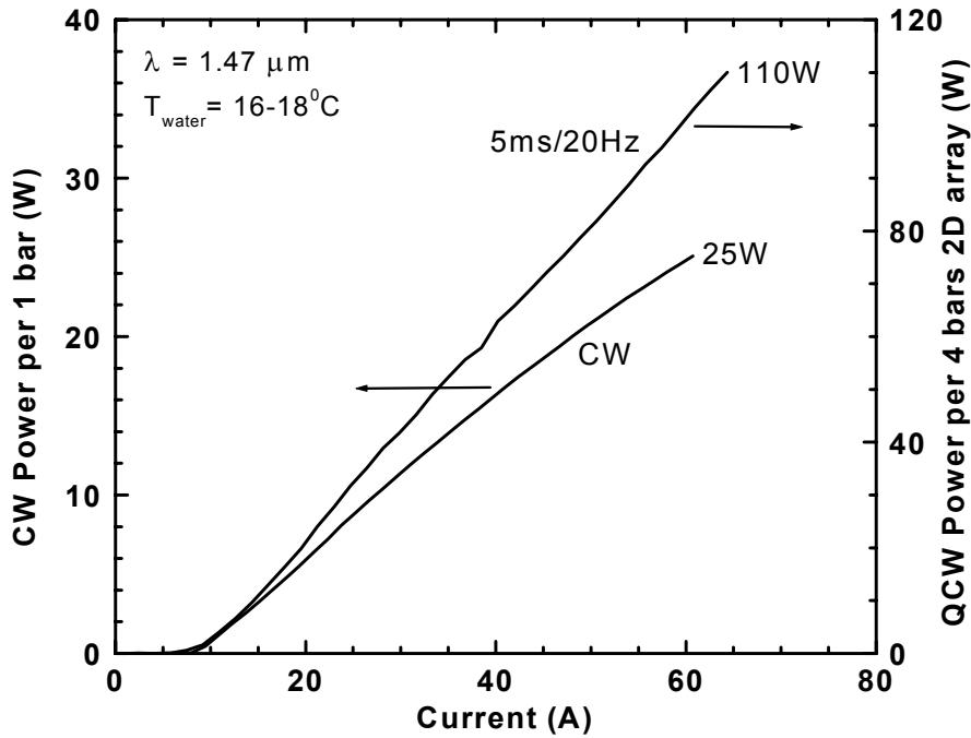
Performance of 1D and 2D  $1.47\mu\text{m}$  laser diode arrays. Array were packaged into microchannel cooled heatsink and operate at CW and QCW conditions.
