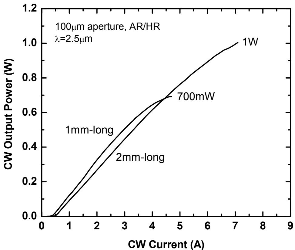
CW performance of high power lasers with broadened waveguide and low internal loss < 4cm<sup>-1</sup>. Devices were In soldered p-side down on water cooled Cu blocks. Water temperature ~ 15°C.
