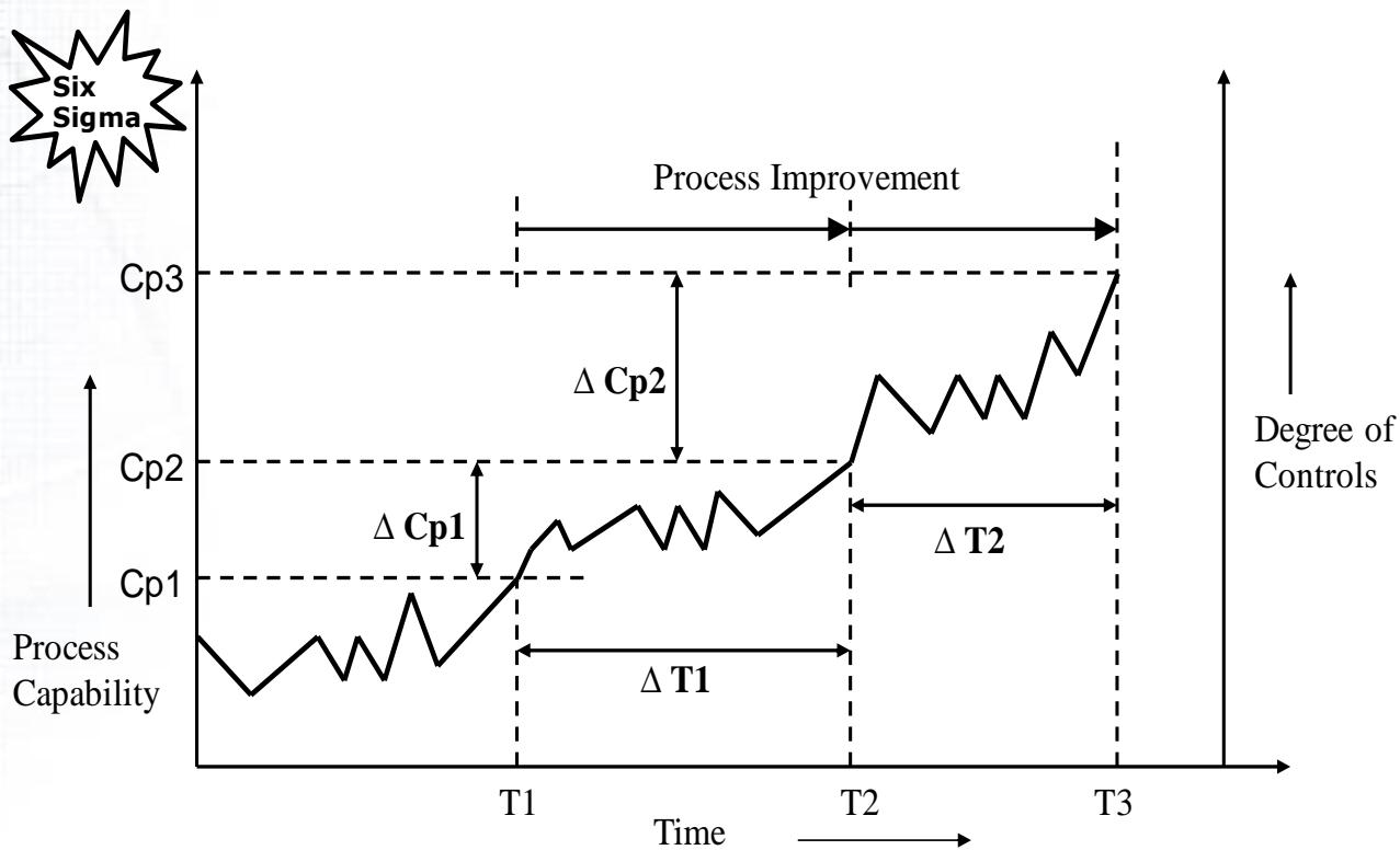
$$\Delta Cp = f(\text{process control} \times \text{process improvement}) \times \Delta T + \text{inherent process variation}$$
