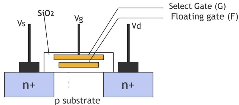
The capacitive coupling between G, F, and substrate is used to regulate the threshold voltage by controlling the charge stored.
