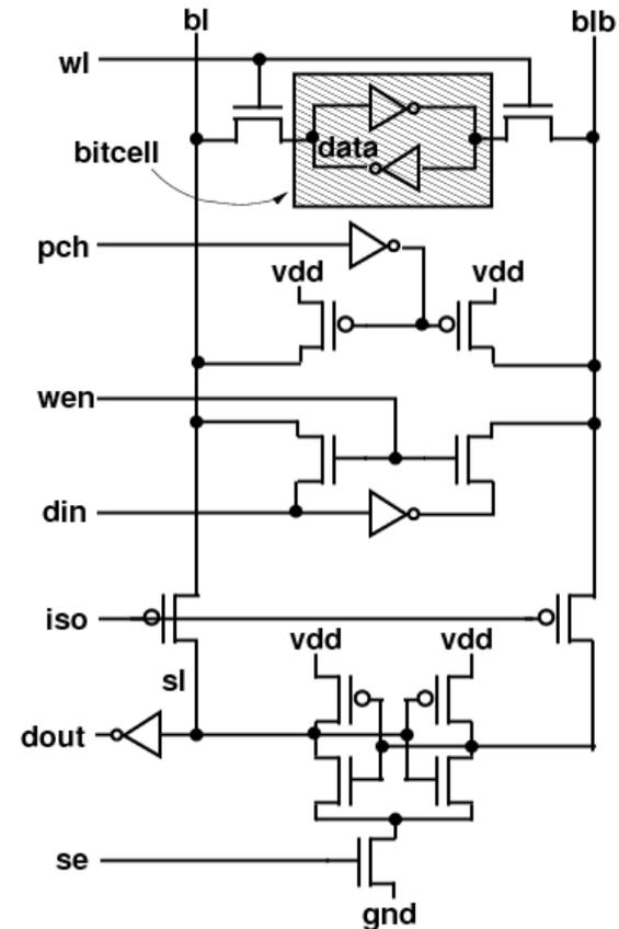
Under the timing constraints for operation the bit cell behavior can be modeled as a state machine.
