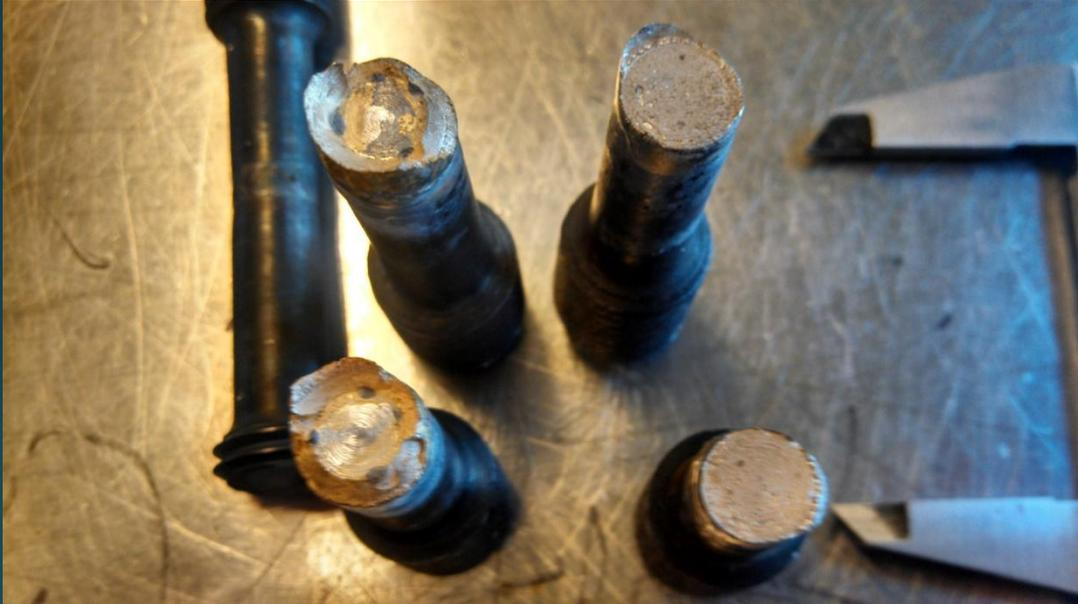
Both the silver solder and braze joints failed.
