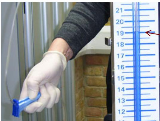
Open the IV fluid bag and slowly fill the manometer to a level higher than the expected CVP
