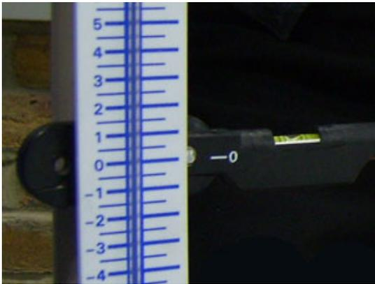
Move the manometer scale up and down to allow the bubble to be aligned with zero on the scale. This is referred to as 'zeroing the manometer'.
