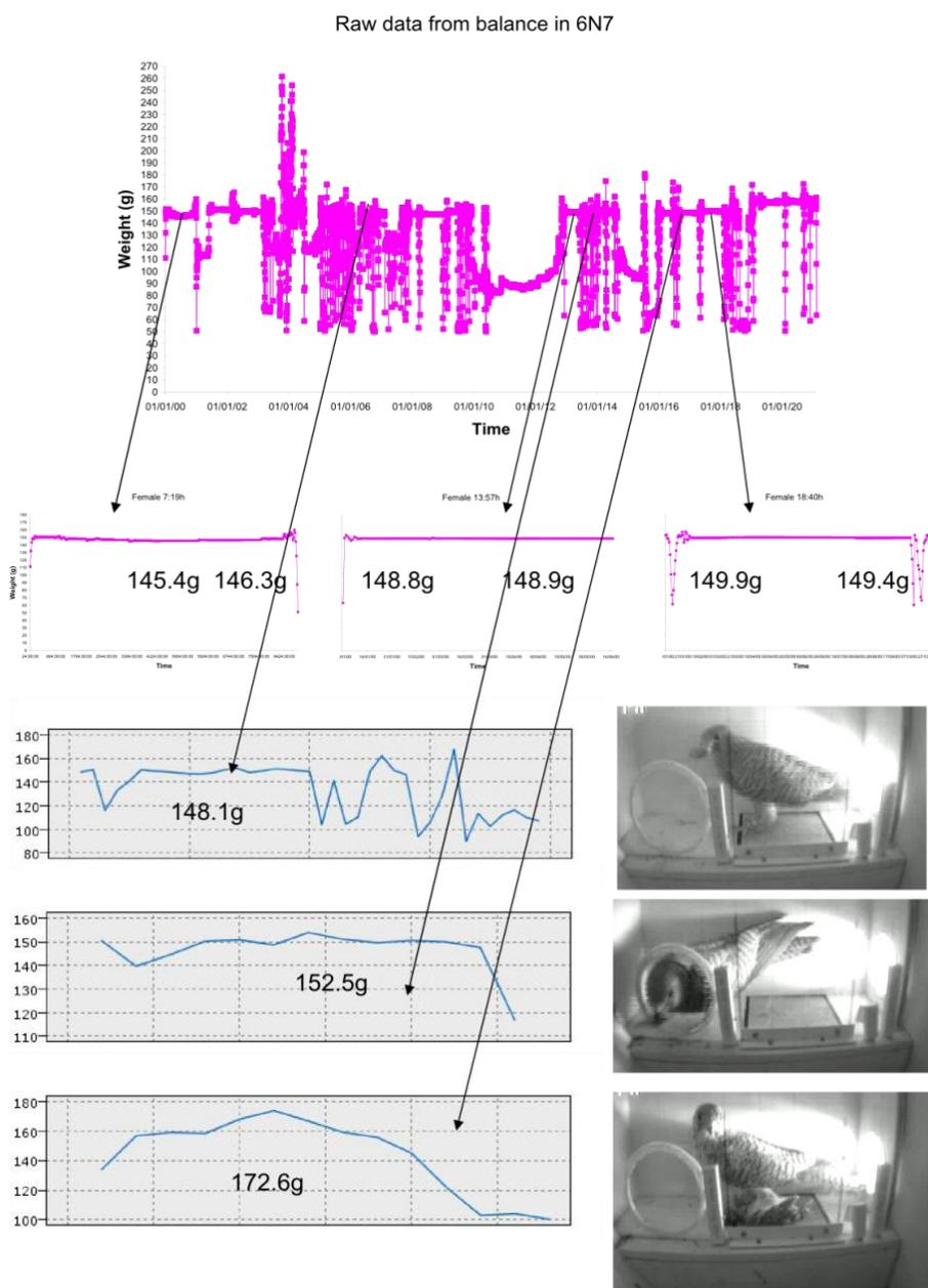
In our results, stable patterns, due to the tare and gain calibration, offer weight estimation with accuracy better than a gram. As can be seen, the system offers an error in the range predicted by the
