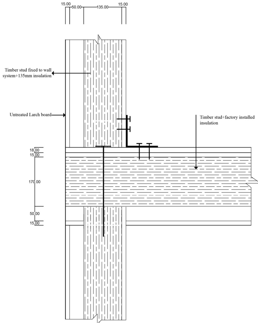
Figure 3. Configuration of the CLT external wall and roofs.
