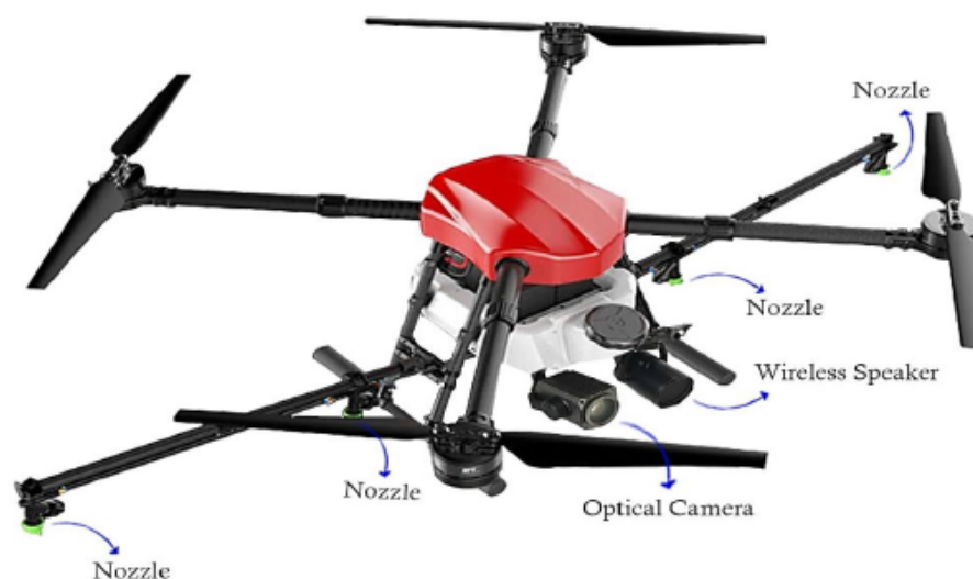
Figure 7. Drone used for spraying disinfectants [62].
