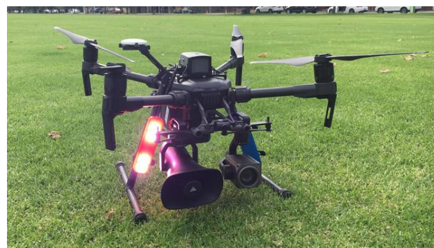
Figure 4. Broadcasting a message by using a loudspeaker [50].
