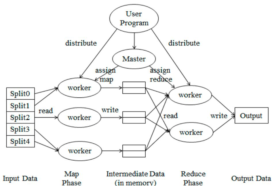
Figure 2. The working principle of Spark.
