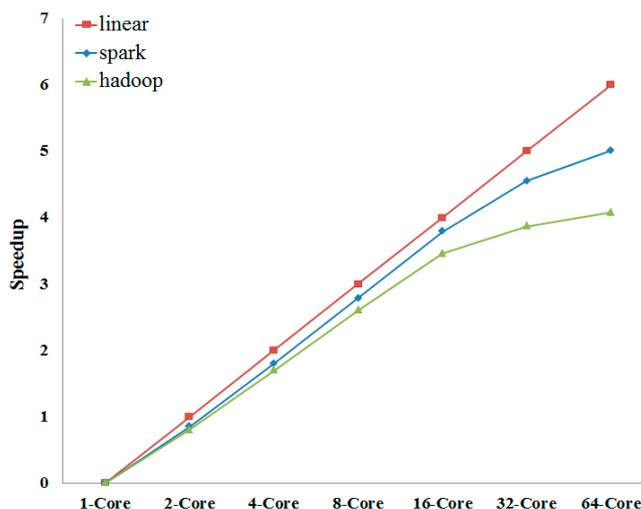
Figure 4. Comparison between the speedups of Spark and Hadoop. In order to make the linear speedup to be a straight line, we let  $y = \log_2(T_1/T_n)$ .  $T_1$  is the running time of common program (single core).
