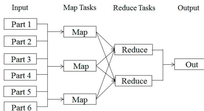
**Figure 1.** The operation process of MapReduce framework.
