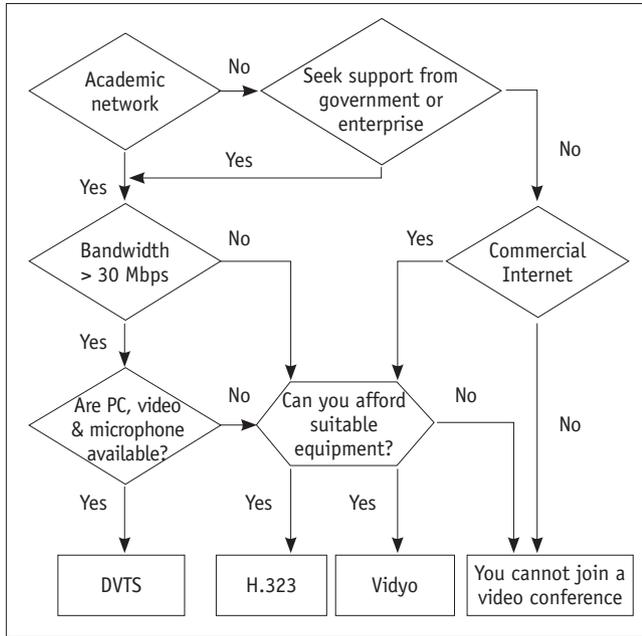
**Fig. 6. Flowchart to assist in correct selection of system.**
