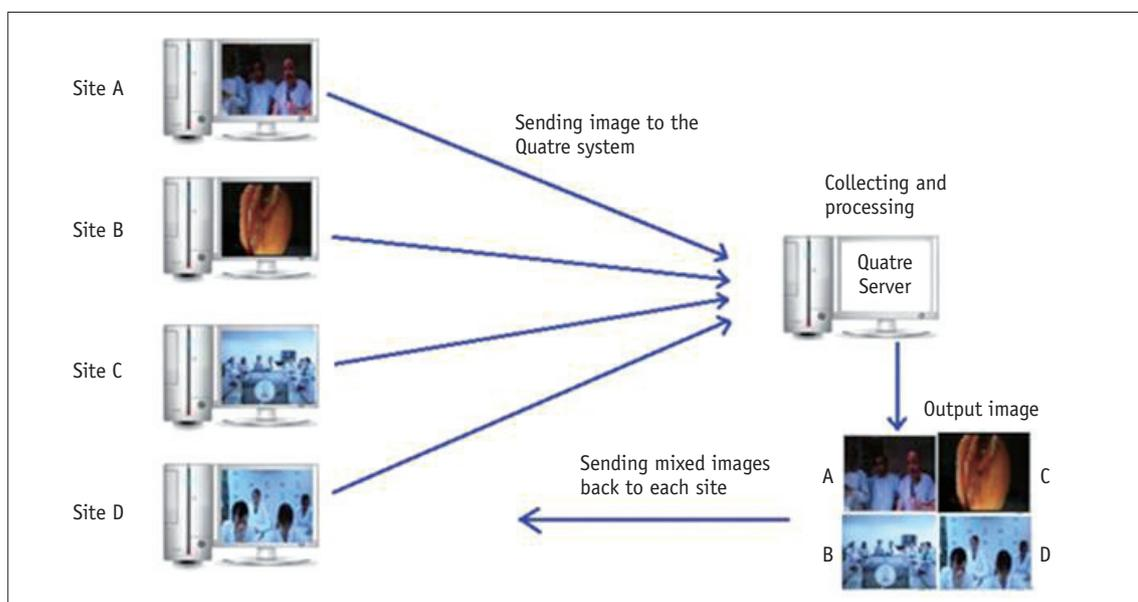
**Fig. 3.** Quatre, multi-point control unit for DVTS. Video image from each site is merged into one image by Quatre server, and is then sent back to original site.
