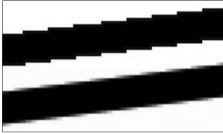
**Fig. 8. Aliasing problem: “aliasing” (top) versus “antialiasing” (bottom).**
