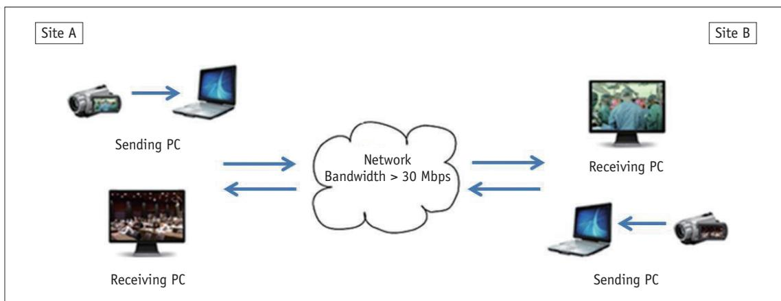
Fig. 1. DVTS system with point-to-point connections.
