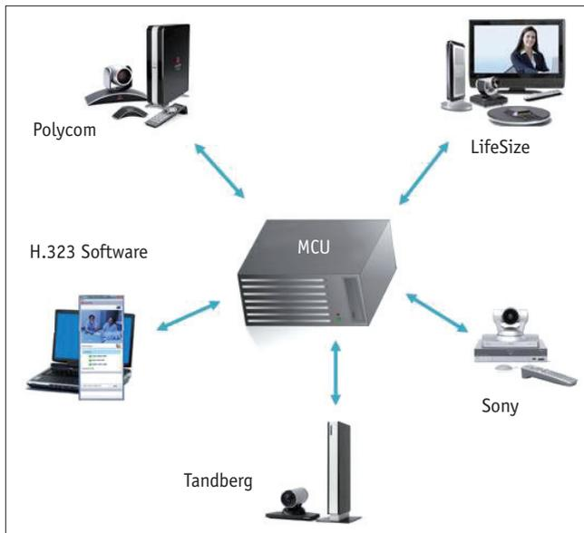
**Fig. 4. H.323 video conferencing system: multi-site connections between different companies using MCU (multi-point control unit).**
