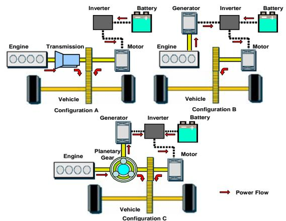
**Figure 1 Hybrid vehicle configurations: A. Parallel; B. Series; C. Power-split**
