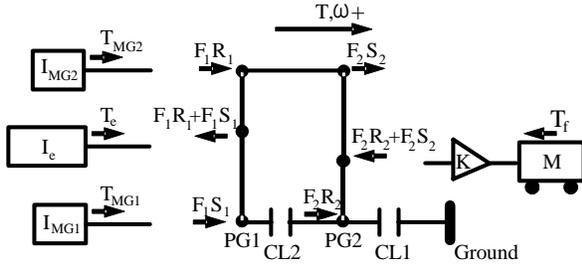
Figure 4 Free body diagram of an example dual-mode power-train
