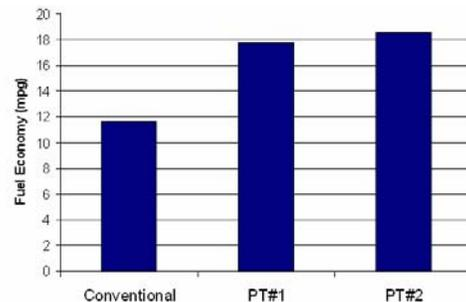
Figure 7 Best performance of the two candidate configurations over the FTP75 cycle using DP optimal control.
