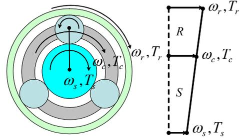
Figure 2 Planetary gear set and the lever diagram
