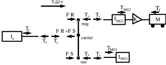
Figure 3 Free body diagram of the THS power-train
