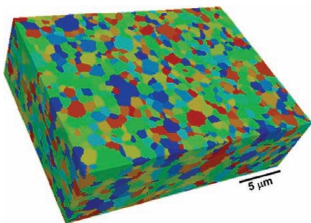
**Figure 12. Reconstructed 43 collected and 280 nm spaced serial sections of EBSD data from undoped yttria [49]. With kind permission from John Wiley & Sons, Inc., *Journal of the American Ceramic Society*, “Characterization of the grain-boundary character and energy distributions of yttria using automated serial sectioning and EBSD in the FIB”, 92 [7] (2009) 1580-1585, S.J. Dillon, G.S. Rohrer, Figure 3.**
