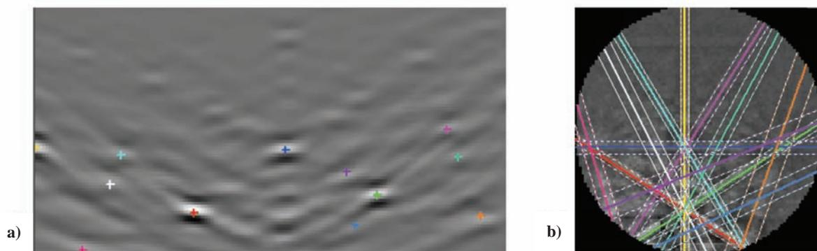
**Figure 5. Kikuchi band detection by Hough transform: a) Hough space, b) detected bands reconstructed from Hough space**
