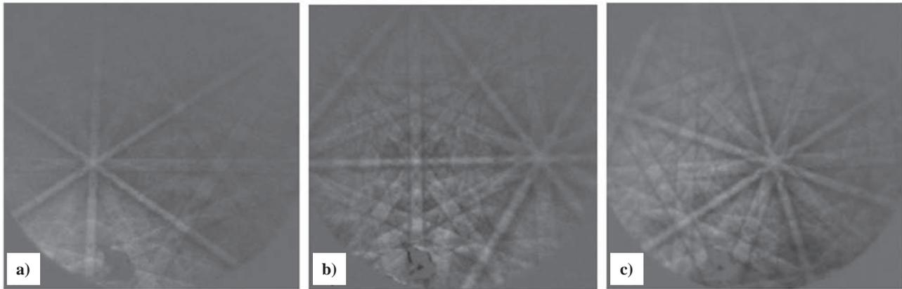
**Figure 4. EBSD patterns from: a) commercially pure aluminium with face-center-cubic (FCC) structure, b) electrical steel (Fe-Si alloy) with body-center-cubic (BCC) structure, c) alpha phase titanium with hexagonal-close-packed (HCP) structure**
