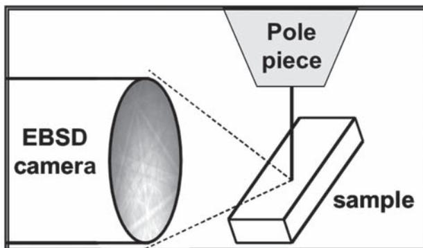
Figure 3. Position of the sample inside the SEM chamber relative to pole piece and phosphorous screen
