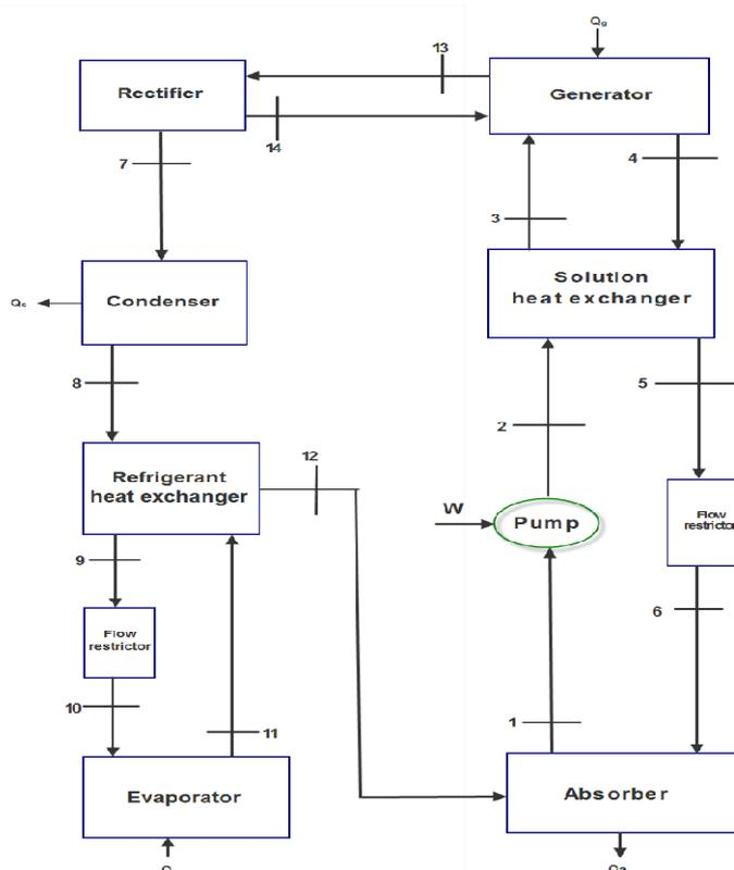
Fig - 1 Ammonia-water absorption refrigeration system flow diagram [12]
