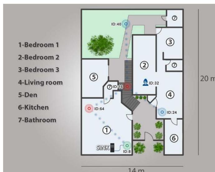
Once the network is formed, communication between the mobile node and the infrastructure can begin and data can be sent. In this test, a person representing a mobile node moved freely throughout the home to determine the number of hops and RSSI. To do this, data packets were generated and routed to the SINK, as shown in Table 5.
