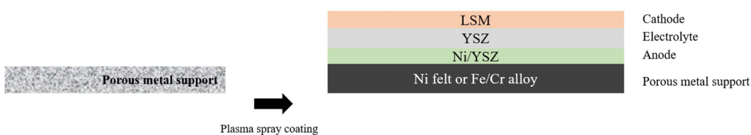
Fig. 4. DLR fabrication process for metal supported cell.
