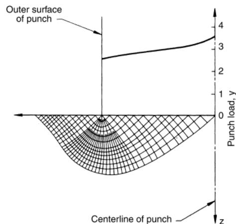
**Fig. 2** Slip-line-field solution for a flat-ended circular punch. Source: R.T. Shield, On the Plastic Flow of Metals Under Conditions of Axial Symmetry, *Proc. Roy. Soc.*, Vol A233, 1955, p 267
