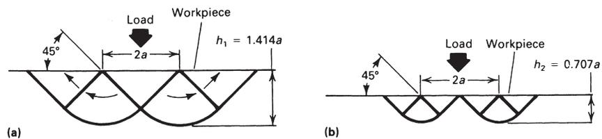
**Fig. 1** Slip-line-field solutions for a flat-ended two-dimensional punch having a width of  $2a$ . (a) Prandtl's flow pattern. Flow in unshaded area is downward and to left and right, as indicated by arrows in shaded areas. (b) Hill's flow pattern. Flow is to left and right in directions indicated by arrows in (a), but is separated. Source: A.R. Fee, R. Segabache, and E.L. Tobolski, Introduction, *Mechanical Testing*, Vol 8, *ASM Handbook*, ASM International, 1985, p 72
