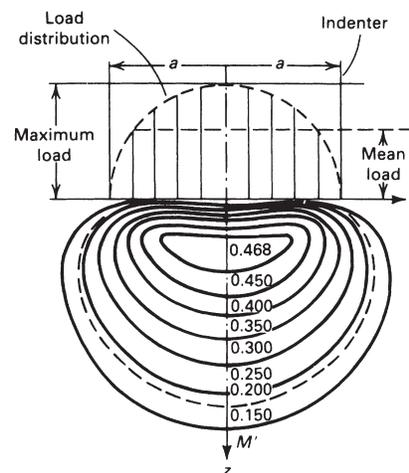
**Fig. 4** Hertz lines of constant maximum shear stress on a meridional plane below the surface of an elastic, semi-infinite body, caused by a frictionless load from a rigid sphere of very large radius.  $M'$  = maximum shear stress in body divided by mean stress (unit load) on the sphere. Source: A.R. Fee, R. Segabache, and E.L. Tobolski, Introduction, *Mechanical Testing*, Vol 8, *ASM Handbook*, ASM International, 1985, p 72
