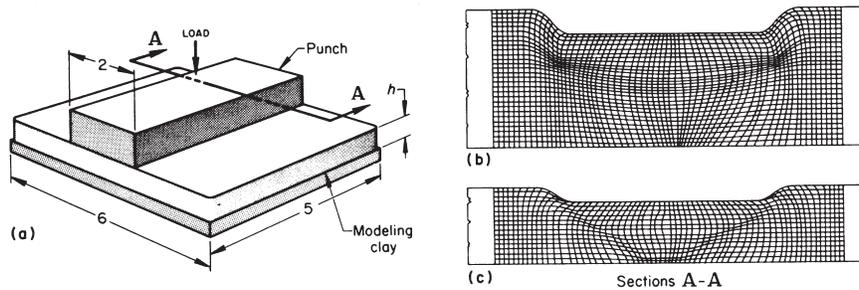
**Fig. 5** Grid patterns on transverse planes of modeling-clay specimens in plane strain by a flat punch. (a) Arrangement for the test. (b) Pattern obtained when  $h = 1.414a$  as in Fig. 1(a). (c) Pattern obtained when  $h = 0.707a$  as in Fig. 1(b). Test specimens of both thicknesses were supported by a rigid steel plate. Source: Hardness Testing, *Nondestructive Inspection and Quality Control*, Vol 11, *Metals Handbook*, 8th ed., American Society for Metals, 1976, p 3
