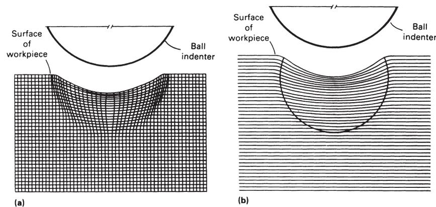
**Fig. 3** Deformed grid pattern on a meridional plane in a Brinell hardness test. (a) Modeling clay. (b) Low-carbon steel. Source: A.R. Fee, R. Segabache, and E.L. Tobolski, Introduction, *Mechanical Testing*, Vol 8, *ASM Handbook*, ASM International, 1985, p 72
