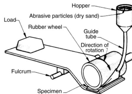
**Fig. 8** Schematic illustration of a dry-sand erosion test used for evaluating resistance to low-stress scratching abrasion. Source: *Wear Failures, Failure Analysis and Prevention*, Vol 10, *Metals Handbook*, 8th ed., American Society for Metals, 1975, p 153
