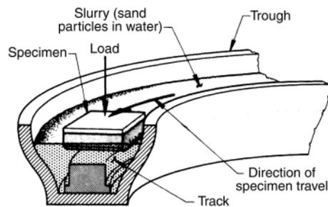
**Fig. 7** Schematic illustration of a wet-sand abrasion test. This is a well-validated wear test simulating high-stress grinding abrasion. Source: *Wear Failures, Failure Analysis and Prevention*, Vol 10, *Metals Handbook*, 8th ed., American Society for Metals, 1975, p 153
