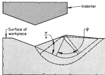
**Fig. 6** Slip-line-field solution for two-dimensional indentation. Solid lines correspond to the frictionless case, where  $\psi = 70$ ; dashed lines correspond to the case with friction. The pattern for a frictionless indenter acting on annealed material will also resemble the dashed line pattern. Source: Hardness Testing, *Nondestructive Inspection and Quality Control*, Vol 11, *Metals Handbook*, 8th ed., American Society for Metals, 1976, p 3
