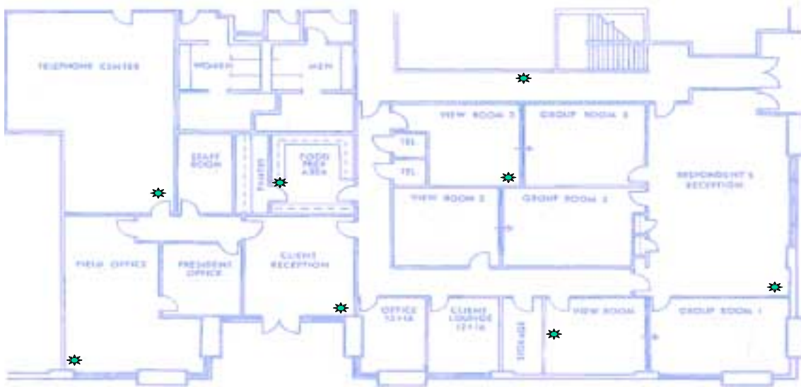
Fig. 1. Four storey building layout with wireless sensors
