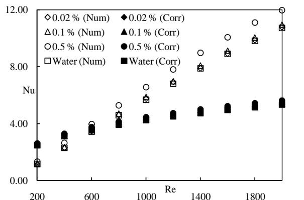
Fig. 6 Effect of volume fraction of  $Al_2O_3$  nanofluid on heat transfer enhancement in the laminar regime
