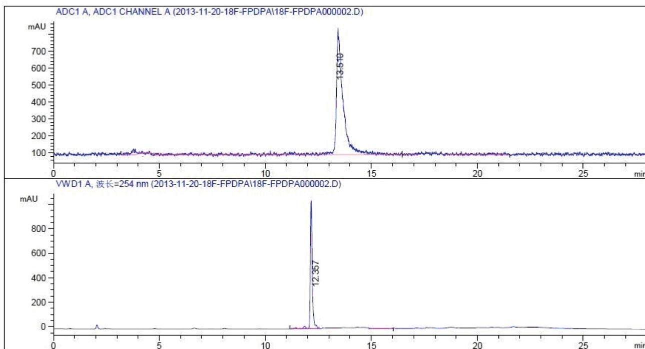
**Figure 1: Typical HPLC-UV chromatograph (bottom) and HPLC-radioactivity detector chromatograph (top) of [<sup>18</sup>F]FP-DPAZn2 solution after purification.**
