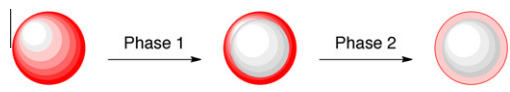
Fig. 8. Schematic representation of biphasic release from bare MSN. Phase 1: fast release from center of MSN. Phase 2: slow release from R6G “skin” [19].
