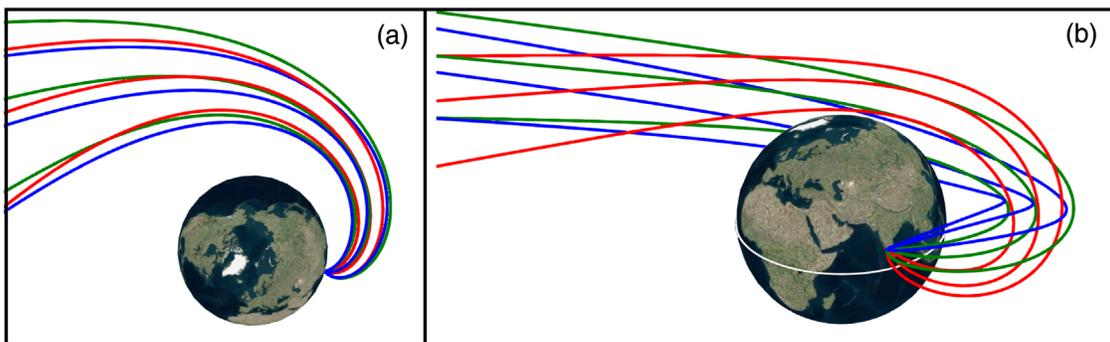
FIG. 4. GCR trajectories near the cutoff rigidity responsible for the burst viewed from the (a) north pole and (b) the equator. NW, N, NE shown in blue, W, V, E in green, SW, S, SE in red.
