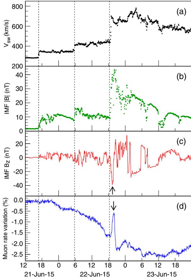
FIG. 1. Top 3 panels show WIND data time shifted to the bow-shock nose: (a)  $V_{sw}$ , (b)  $|B|$ , (c)  $B_z$ , (d) GRAPES-3 muon-rate. Vertical dashed lines indicate CME arrival times (UT).
