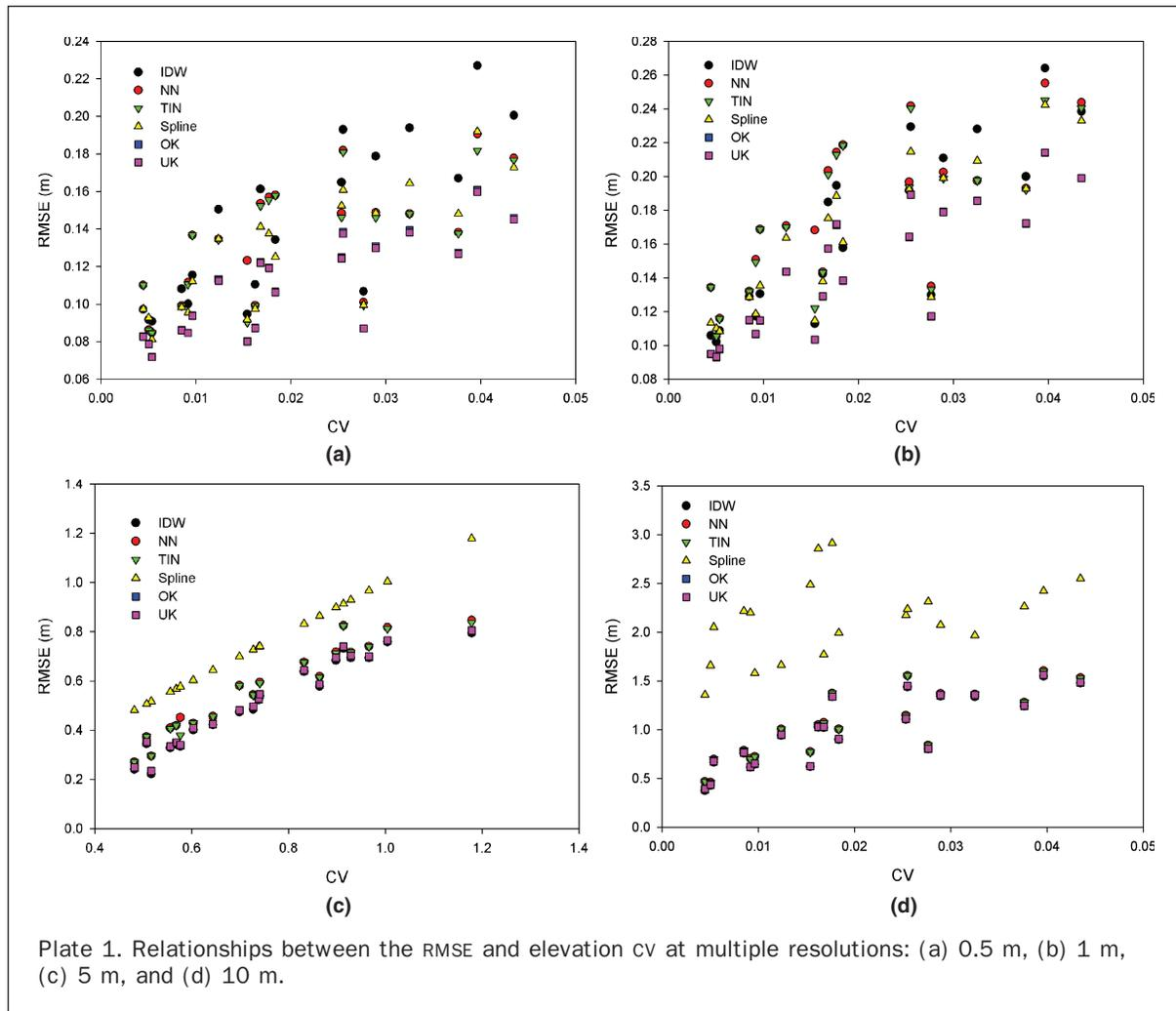
Plate 1. Relationships between the RMSE and elevation CV at multiple resolutions: (a) 0.5 m, (b) 1 m, (c) 5 m, and (d) 10 m.
