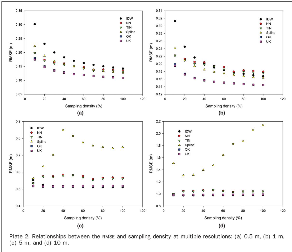
Plate 2. Relationships between the RMSE and sampling density at multiple resolutions: (a) 0.5 m, (b) 1 m, (c) 5 m, and (d) 10 m.
