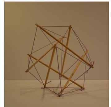
**Fig. 7** Tensegrity icosahedron: Full - External force applies – resilience (Self-build model)
