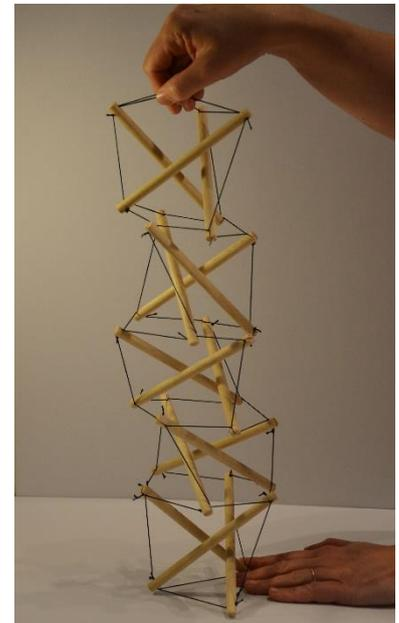
**Fig. 6** Basic tensegrity mast, Notice the similarity with the segmented spine (Self-build model)
