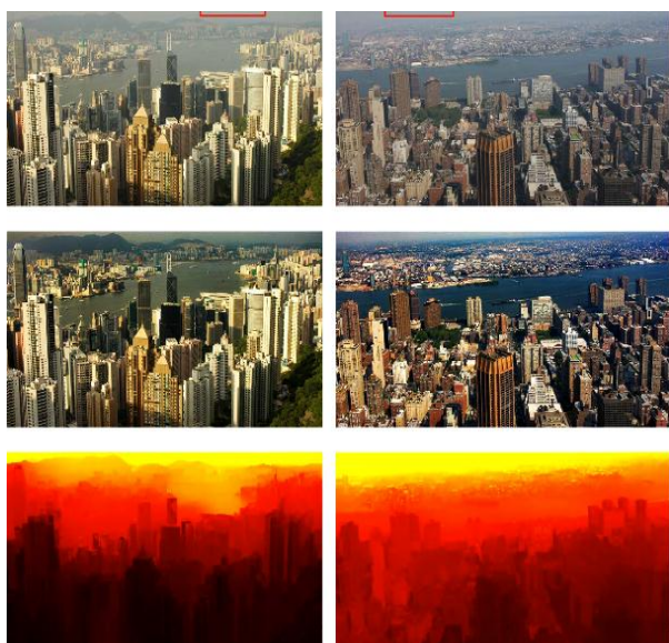
Fig 2 Haze removal results. Top: input haze images. Middle: restored haze-free images. Bottom: depth maps.
