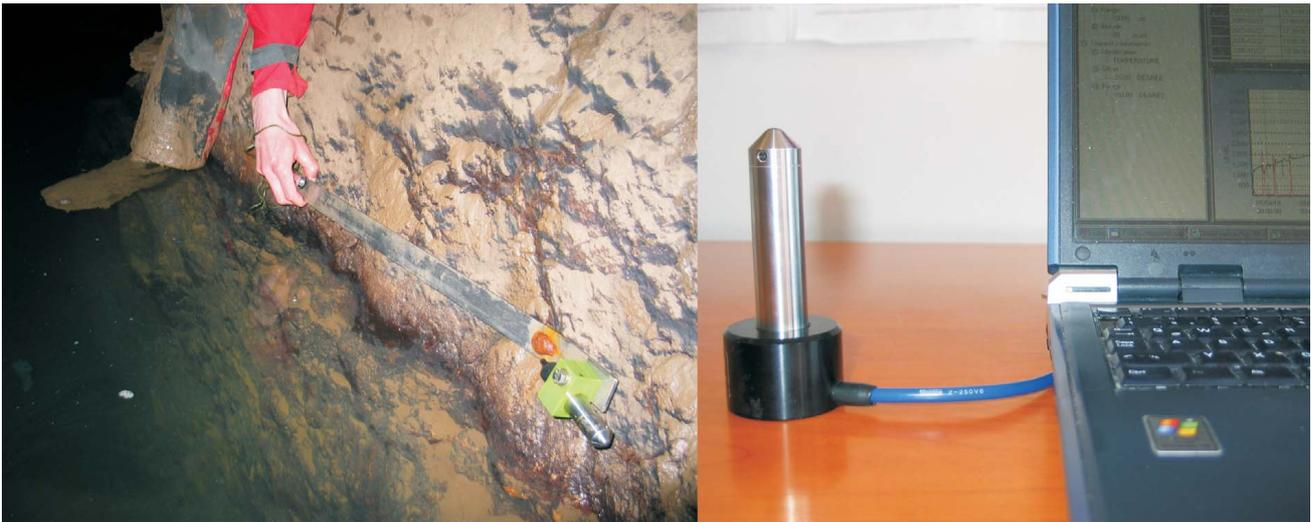
Figure 2: Data logger in a cave (left) and connected to a PC via optical bridge (right).
