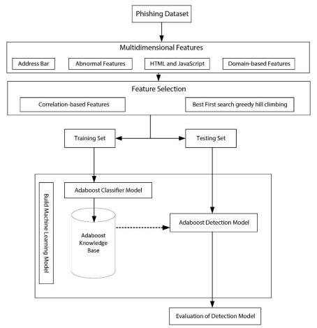
Figure 1. PhiBoost structure.
