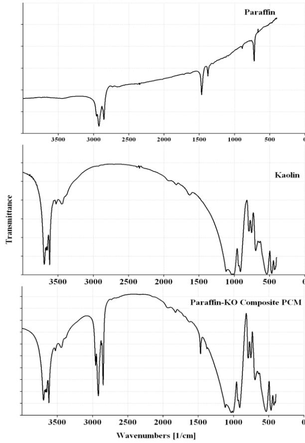
Figure 4. FT-IR spectra of Paraffin, Kaolin and Paraffin-Kaolin composite PCM.
