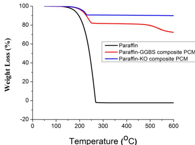
**Figure 7.** TGA thermograms of the paraffin and CPCMs.
