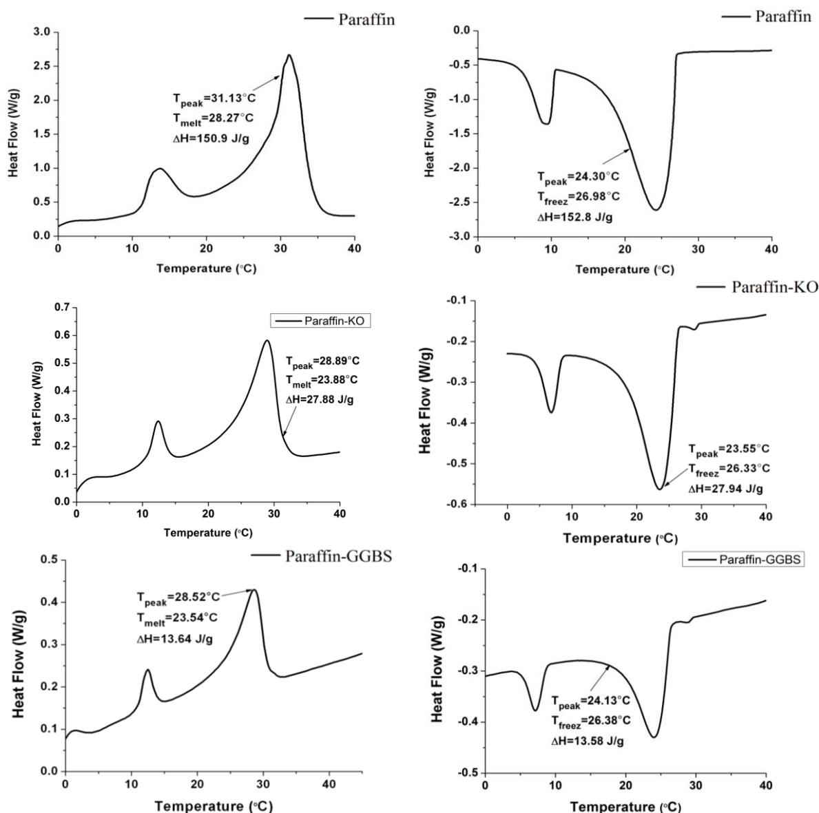
Figure 6. DSC thermograms of the paraffin and CPCMs.
