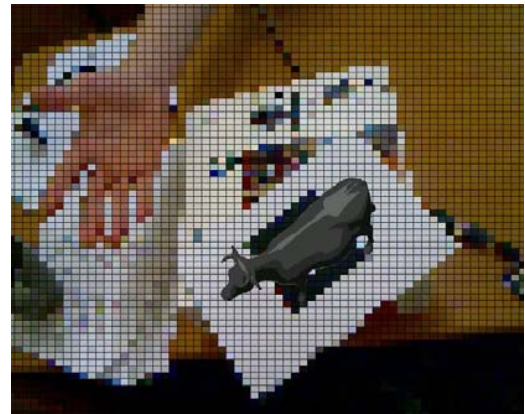
Figure 10: Geometry-based technique: cartoon shading, Image-based technique: tile Effect
