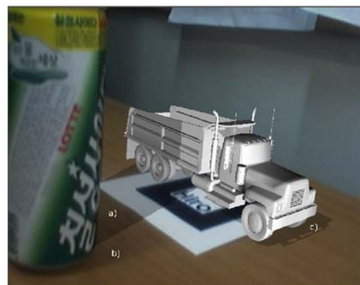
Figure 6: Shadows of virtual and real objects: a) shadow from the phantom objects, b) real shadow of the can, c) shadow of the truck
