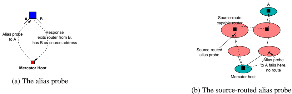
Fig. 3. Repeated alias probing can resolve router aliases. In some cases, source-routed alias probes are necessary for alias resolution.
