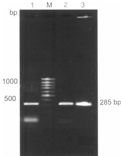
Fig. 1—Amplification of 285 bp DNA fragment by G1/G2 specific PCR from serum and liver samples of representative experimentally infected guinea pigs. [Lane M, 100 bp DNA ladder; Lane 1, Canicola DNA taken as control positive; Lane 2, serum sample; Lane 3, liver sample]
