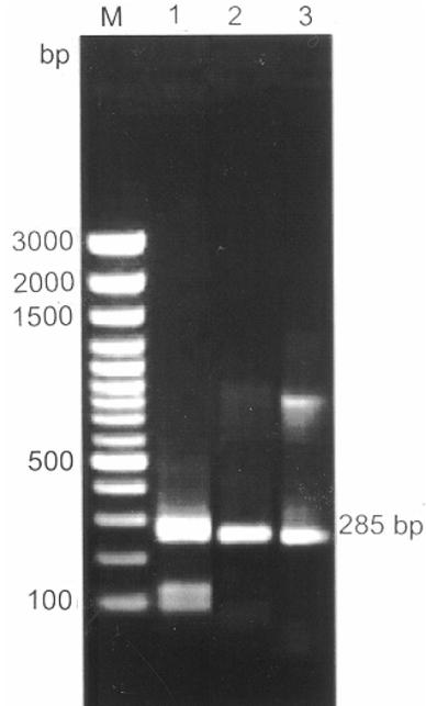
Fig. 6—Amplification of 285 bp DNA fragment by G1/G2 specific PCR from field samples. [Lane M, 100 bp DNA ladder; Lane 1, serum sample (S23) from cattle; Lanes 2 and 3, liver (L19) and kidney (K10) samples, respectively, from buffaloes]
