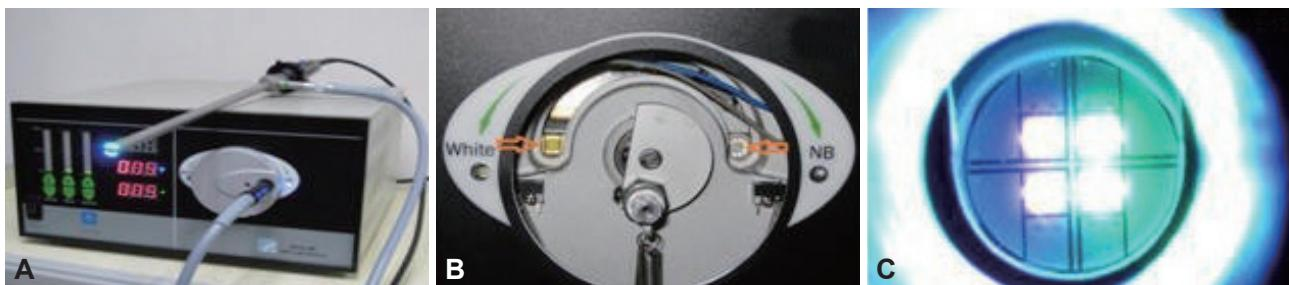
**Fig. 2.** (A) Light-emitting diode (LED)-narrow band imaging light source PR650, cursors for 0% to 100% white, green/blue light mix. (B) Left  $\Rightarrow$ : white LED chip; right  $\Leftarrow$ : green/blue LED chips. (C) Close-up view: green/blue LED chips.
