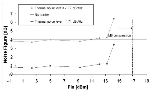
Fig 6(b). Variation of NF with input power for the amplifier in figure 6(a).
