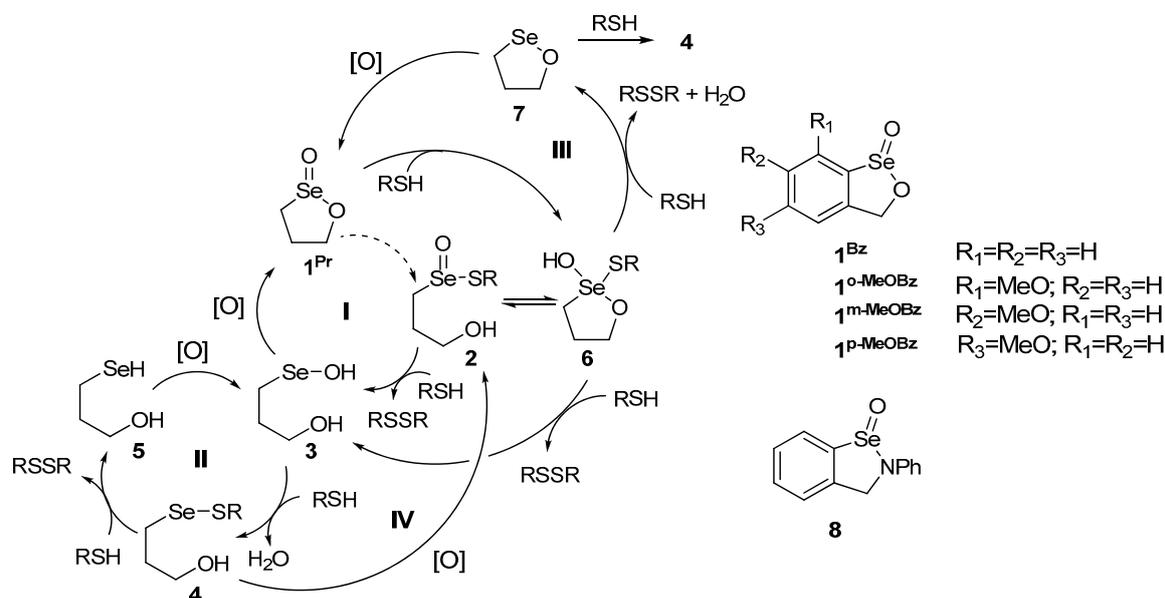
**Scheme 1.** Mechanisms for ROS scavenging for five-membered cyclic seleninates such as **1<sup>Pr</sup>** and **1<sup>Bz</sup>**.
