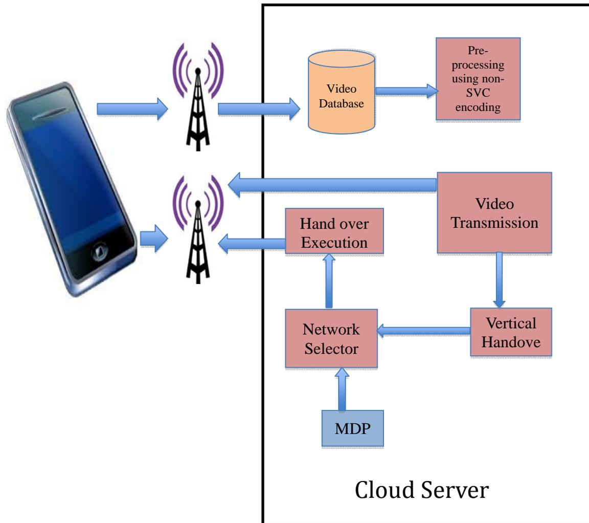
Fig. 1 Real-Time Multimedia Streaming Architecture
