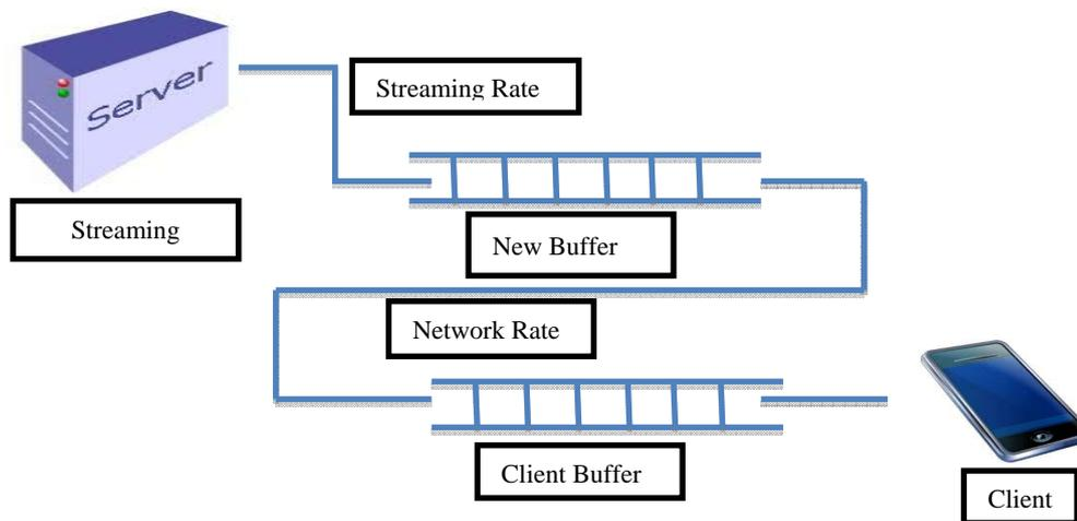
Fig.2 Adaptive Video Streaming Flow Diagram
