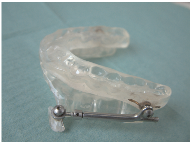
Figure 2. Acrylic breakage on the lateral telescopic attachment.
