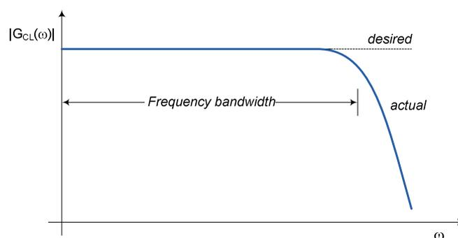
Fig. 2. The closed-loop amplitude (magnitude) response over frequency.
