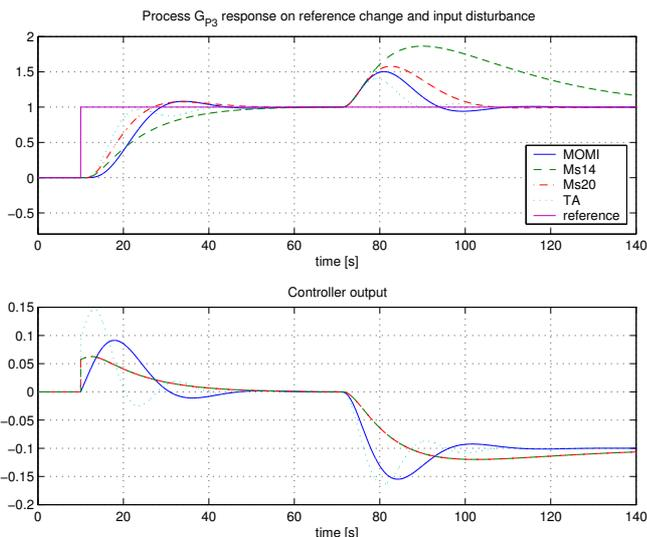
Fig. 5. Closed-loop response of the process  $G_{P3}$  with PI controllers tuned by MOMI, Ms14, Ms20 and TA method.
