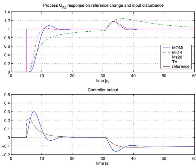
Fig. 4. Closed-loop response of the process  $G_{P2}$  with PI controllers tuned by MOMI, Ms14, Ms20 and TA method.
