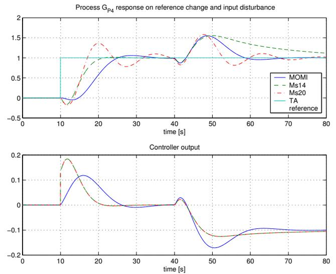
Fig. 6. Closed-loop response of the process  $G_{P4}$  with PI controllers tuned by MOMI, Ms14 and Ms20 method.
