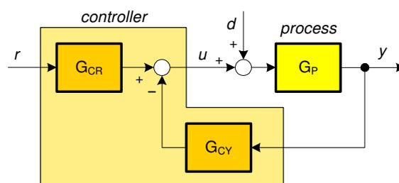
Fig. 1. Typical closed-loop configuration using a 2-DOF controller.
