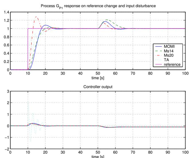
Fig. 3. Closed-loop response of the process  $G_{P1}$  with PI controllers tuned by MOMI,  $Ms14$ ,  $Ms20$  and  $TA$  method.
