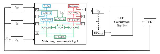
**Figure 8.** The framework of the study on system matching parameters with EEDI under consideration. <sup>1</sup>'a' dashed line means that not in all cases  $SFC_{ME}$  is obtained from SFC curve at a specific engine power. <sup>2</sup>'b' dashed line means that the ship effective power optimization, i.e., the ship hull optimization, is outside the scope of this paper.
