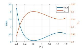
Figure 7. The relationship of EEDI and open water propeller efficiency with different pitch ratios.
