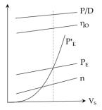
**Figure 3.** Point of intersection of  $P'_E - V_S$  curve and  $P_E - V_S$  curve is the desired speed.
