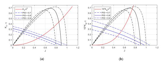
**Figure 2.** Water diagrams under two constraints. (a) Case 1 with  $K_T/J^2$  as a constraint and (b) Case 2 with  $K_O/J^3$  as a constraint.
