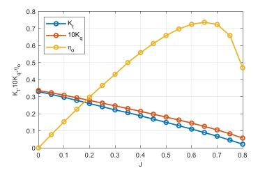
Figure 5. Open water diagram (courtesy of Shanghai Merchant Ship Design and Research Institute).
