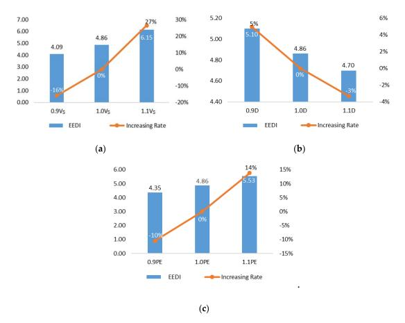
**Figure 10.** Extent of variation of EEDI under different situations of ship speed, propeller diameter and ship effective power: (**a**) with ship speed as a variable; (**b**) with the propeller diameter as a variable and (**c**) with the ship effective power as a variable.
