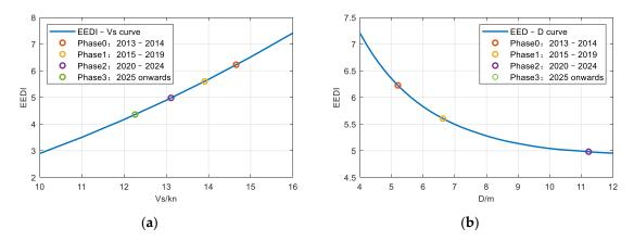
**Figure 12.** The value of key system matching parameters satisfying EEDI of different phases. (**a**) ship speed and (**b**) propeller diameter.
