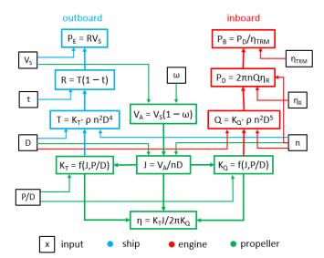
Figure 1. Framework of ship–engine–propeller matching.
