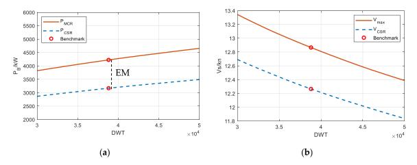
**Figure 13.** The required engine power and ship speed to satisfy EEDI: (**a**) engine power and (**b**) ship speed.
