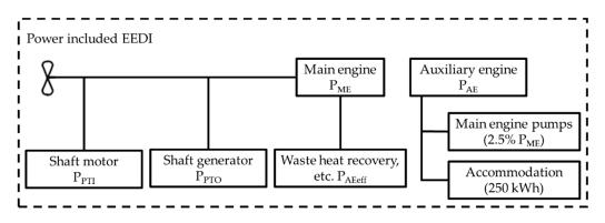
Figure 4. The power involved in the calculation of energy efficiency design index (EEDI).
