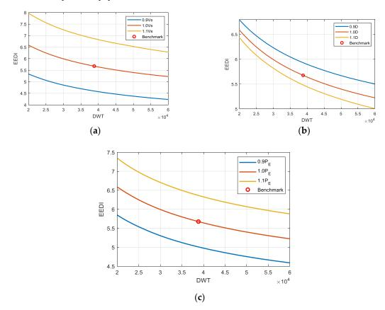
**Figure 9.** EEDI varies with deadweight tonnage (DWT) under different situations of ship speed, propeller diameter and ship effective power: (**a**) with ship speed as a variable; (**b**) with the propeller diameter as a variable and (**c**) with the ship effective power as a variable.
