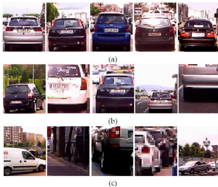
**Figure 8.** Example results: (a) positive hypotheses, (b) hypotheses corresponding to vehicles incorrectly framed; and (c) false positives corresponding to non-vehicles or vehicles out of system's scope.
