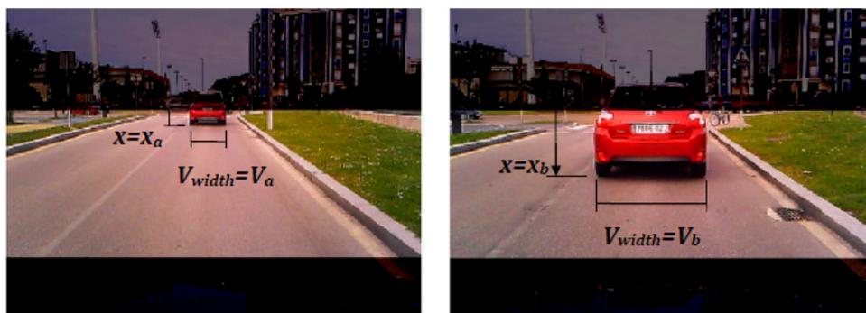
**Figure 4.** Variation of the width of a vehicle according to the vehicle vertical location in the image.
